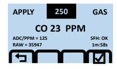
Apply the target gas value shown on screen until RAW ADC stabilizes. A minimum time of 2-3min is recommended. For oxygen sensors, use zero air (20.9% oxygen balanced in N<sub>2</sub>) instead.
