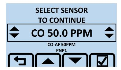
In case of a multigas monitor, the up and down arrows will allow the user to scroll through the different sensors attached. Once the user has selected the sensor that needs calibration, the check mark will take the user to begin calibration:
