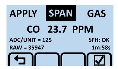
If the calibration is successful and passes all the internal checks, a window will be displayed indicating
