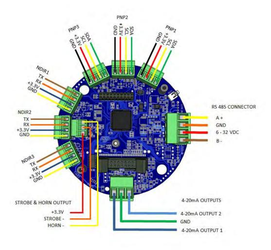
If the expansion board is used, you get the following wiring diagram:
